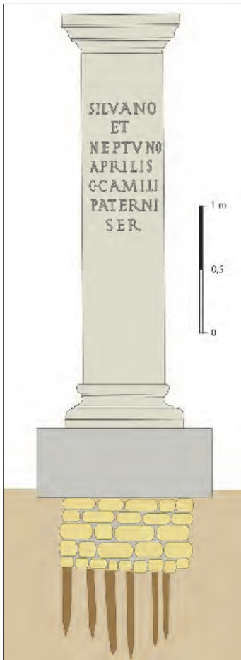
Fig. 164 – Inscribed base of a statue excavated uphill from the canal in 1990. The monument comprised several elements. The limestone column stood on a sandstone cube which, in turn, rested on an underground foundation of masonry. Vertical oak piles, under the foundation, partially preserved at the moment of the excavation, ensured the monument's stability. The original statue on the column has disappeared. SILVANO ET NEPTVNO APRILIS C. CAMILLI PATERNI SER(vus)
