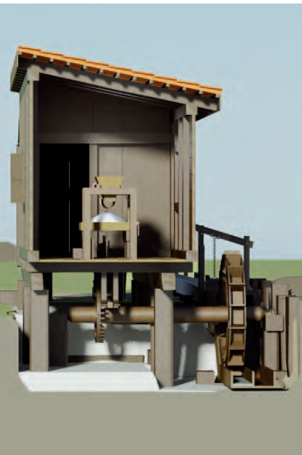
Fig. 172 – Cross-section of the Tourbières watermill. The milling room housing the millstones is on a platform. The gearing mechanism, under the floor of the platform, is driven by the waterwheel (right).
