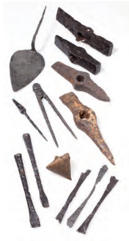
Fig. 36 – Assortment of tools used in different trades related to construction (trowel, hammers, picks, drill bit, compass, plumb line, chisels and spatulas).
