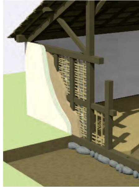
Fig. 125 – The remains of the oldest houses of Aventicum are very poorly preserved. The two pictures taken in insula 15 in 2013 correspond to two successive excavation layers of the same house. The wooden beams (left) of the base of the walls (now carbonised) rested on a stone foundation (right). The drawing above illustrates the mode of construction.
